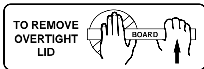
Figure 5 – Use a pry bar or board as shown to remove tight lid.
