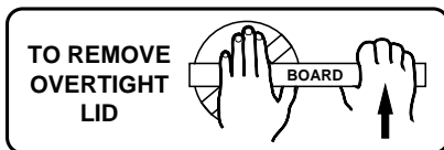
Figure 4 – Use a pry bar or board as shown to remove tight lid.
